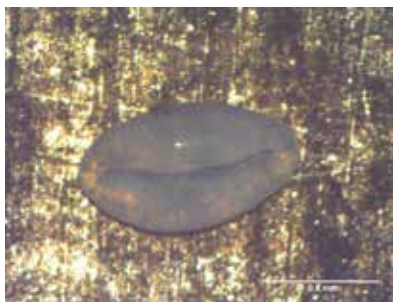
Figure 1. Fumed silica particle dried from suspension on superhydrophobic surface
