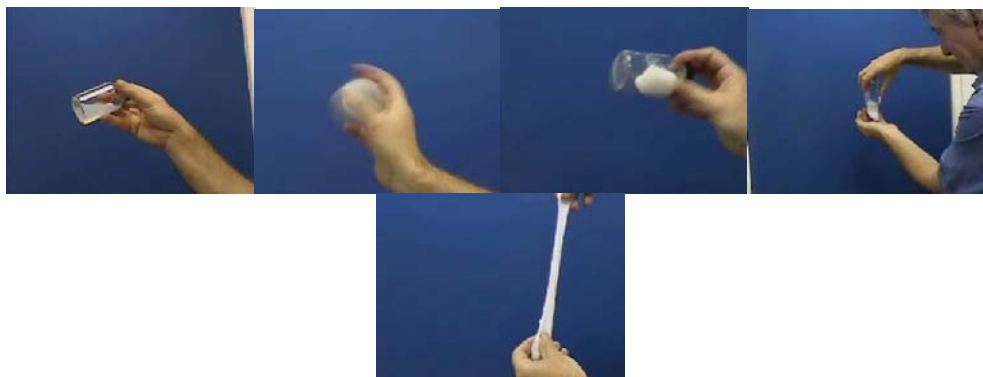
Figure 1 The formation of a shake gel, by simply shaking the formulation which then transforms from a viscous liquid to an elastic solid
