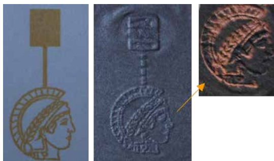
Fig. 1 Preparation of the patterned electrode, from left to right: printed iron-based ink on paper, after thermal treatment to convert the ink into carbon/ceramic arrays, and after metal deposition.
