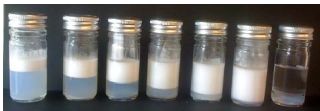
Fig. 1: O/w emulsions of diisopropyladipate oil stabilized by 4% Ludox TM AS40 for increasing amounts of oil from 10% to 70%. Emulsification was successful up to 60% oil and failed at 70%.
