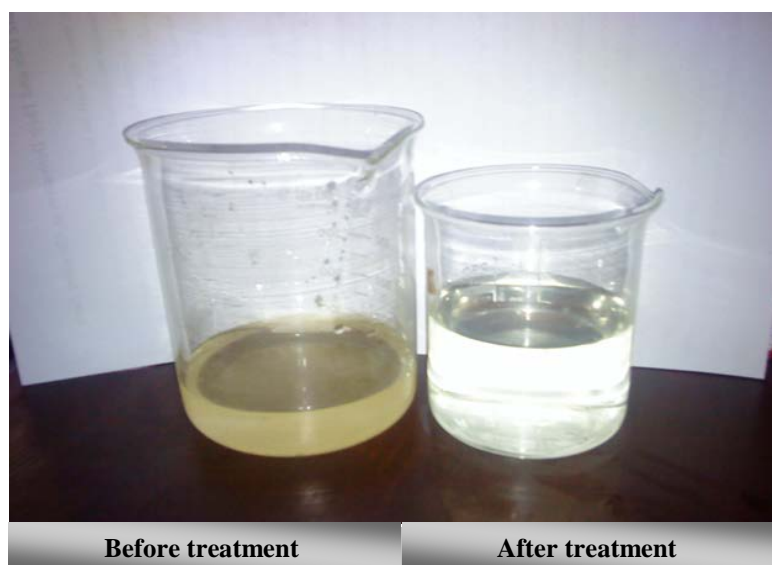
Figure 1: Effect of OD3 on condensate oil-water emulsion at 25 °C.
