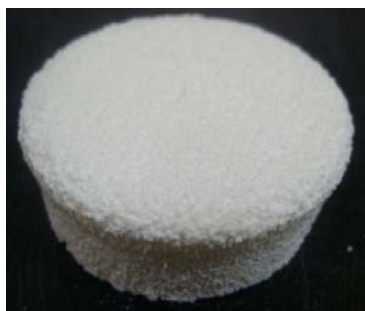
Fig. 1 Photo of dried foam, formed from CAPB-silica dispersions at pH=8.5.
