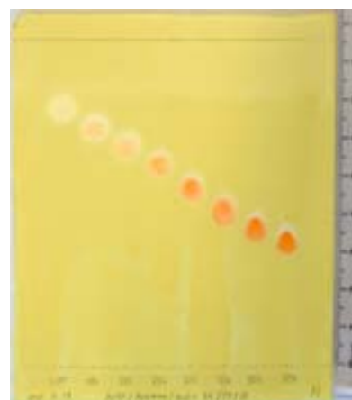
Fig. 1 TLC measurement of the series of pure polyoxyethylene-type nonionic surfactants using the normal phase plate. The spots are placed downward with increasing the EO chain length.
